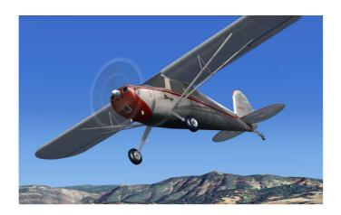
The C140 is a two-seater, single-engine, light utility airplane with a maximum speed of 109 knots (125 mph), never to exceed 122 knots. Original models came equipped with 85-90 horsepower, 4-cylinder piston engines. The C140 was first introduced in 1946 at the end of World War II, and produced from 1946-50. More than 7.664 airplanes have been sold.
