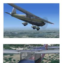
It is a four-seat, single-engine, high-wing airplane, capable of cruising at 131 knots. Original models shipped with 0-300, 145 horsepower, 6-cylinder engines. The C172 is considered the most popular flight training airplane in the world and is still being produced today. More than 35,000 aircraft have been built.
