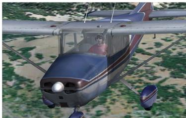
It is a four-seat, single-engine, high-wing airplane, capable of cruising at 131 knots. Original models shipped with 0-300, 145 horsepower, 6-cylinder engines. The C172 is considered the most popular flight training airplane in the world and is still being produced today. More than 35,000 aircraft have been built.
